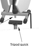
Tripod quick connect socket for quick connect pin
